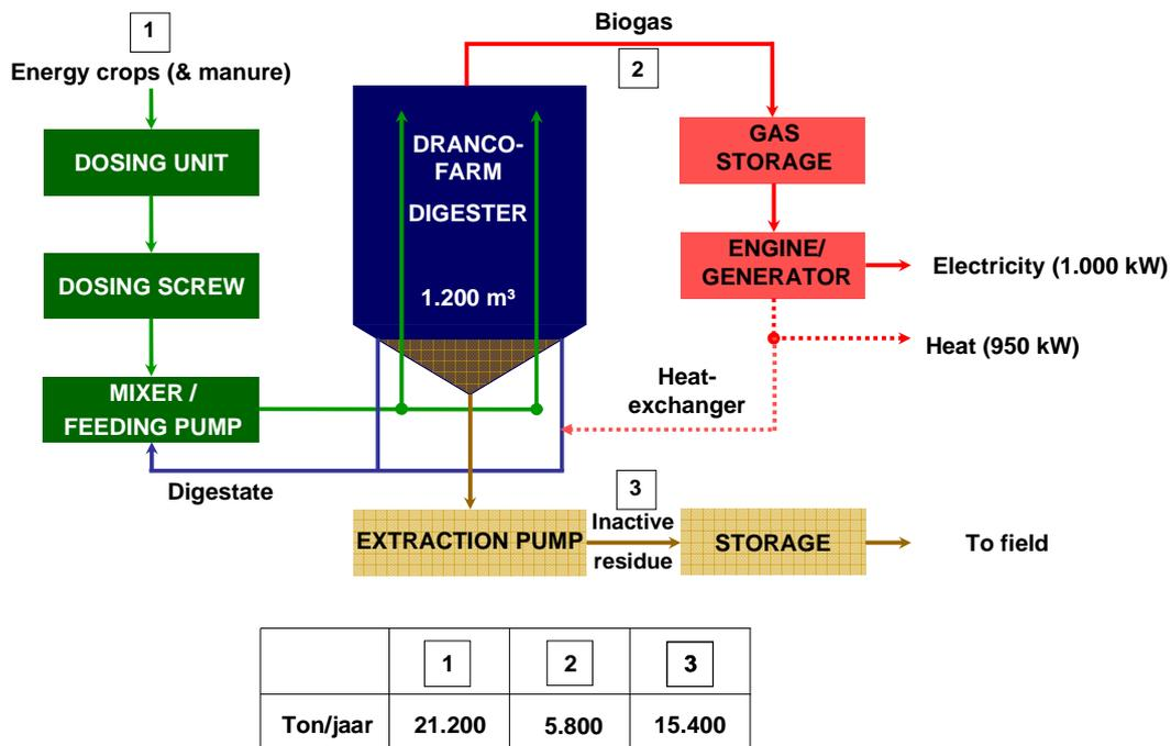
Figure 7: Flow scheme of DRANCO-FARM plant for the digestion of energy crops in Nüstedt (Germany)
