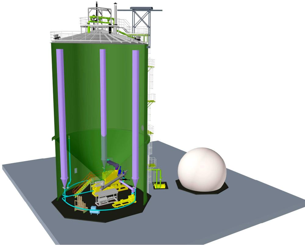
**Figure 2: View of a Dranco digester with internal feeding tubes and with feeding pump under the digestion tank**
