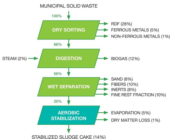
Figure 6: Sordisep for maximum recovery of recyclables and landfill diversion
