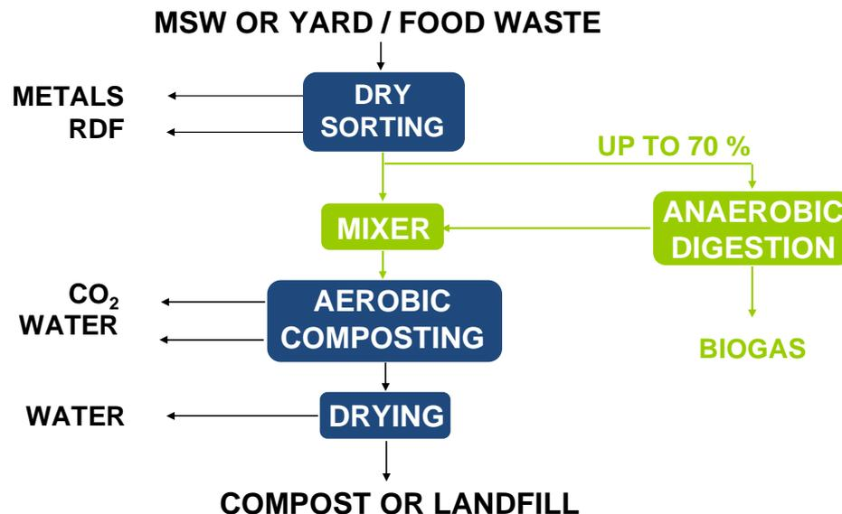
Figure 4: Partial stream digestion
